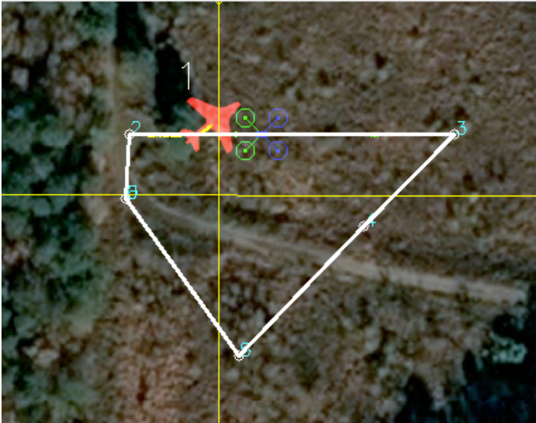
Figure 3: Detail of MAVProxy showing an aircraft, maneuvering to avoid a collision with an intruder. Copilot-generated C code is used by a cFS application to monitor the collision avoidance logic and report property violations.
