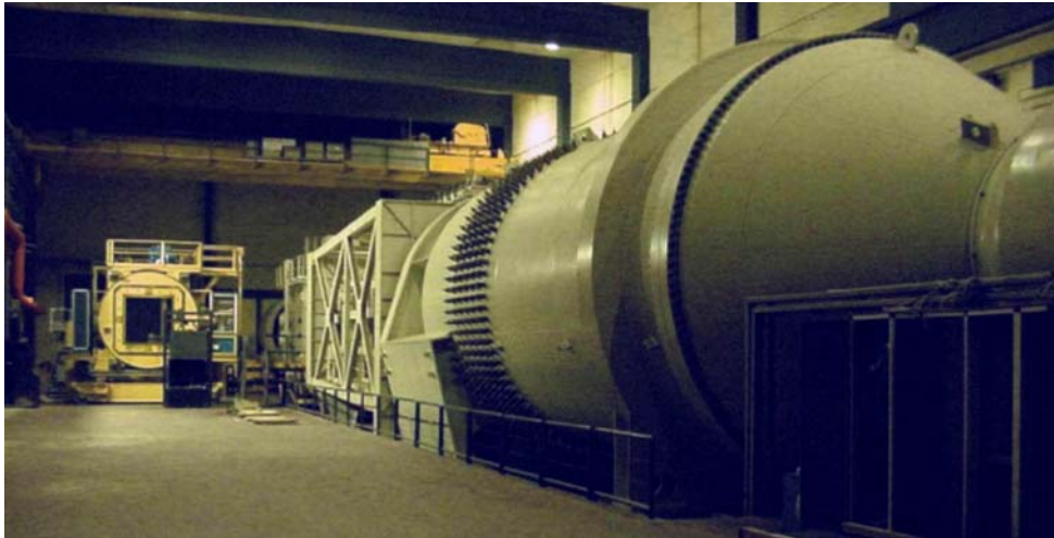
Figure 1. T-38 hall. T-38 is a blowdown-type wind tunnel with 1.5 \times 1.5 \text{ m} and 0.38 \times 1.5 \text{ m} test sections and transonic Mach number range (0.2 to 4). It is driven by air stored in 2600 \text{ m}^3 tanks charged to 20 bars pressure by a 4 MW compressor.
