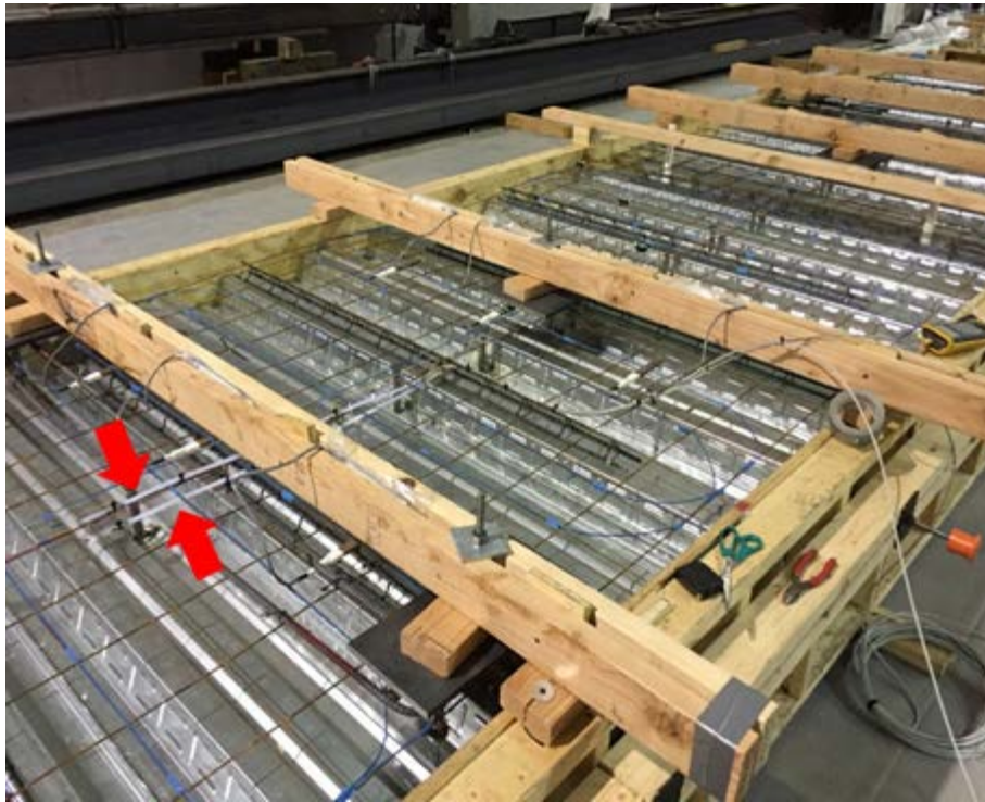
Figure 4-17 Fiber Bragg Grating sensors in CB-DA-AMB indicated by red arrows.
