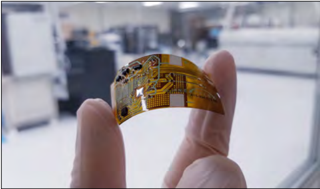
The NextFlex Microcontroller is thin and conformable to most shapes. Credit: NextFlex
