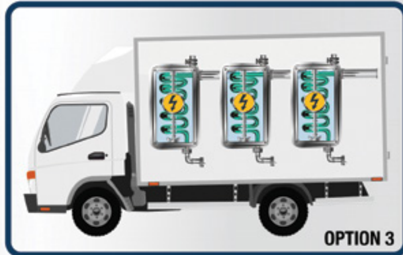
Figure 45. Modular chemical process intensification (MCPI) provides a new paradigm for leaner, greener, cleaner, and safer manufacturing. MCPI uses standardized modular components and other hardware prototypes to increase efficiency and flexibility while reducing costs. MCPI reactors can be used in a variety of configurations as single units (option 1), in different combinations (option 2), and even as portable systems (option 3). Credit: RAPID
