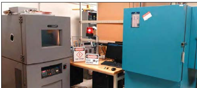
High-temperature ovens for SiC power device accelerated stress tests at Texas Tech University. Credit: PowerAmerica.
