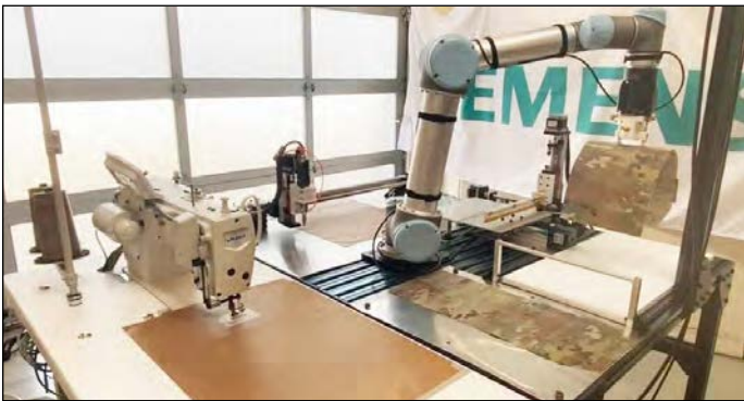
A demonstration of the first ROS (robotic operating system) controlled industrial sewing machine to make military uniforms in a project led by Siemens.
