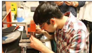
PowerAmerica short course student assembling WBG power semiconductor devices into a module. Credit: PowerAmerica
