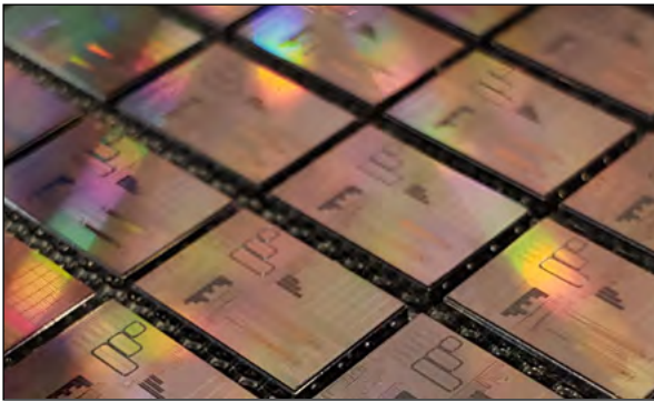
Photonic Integrated Chips from AIM Photonics 300 mm MWP programs ready to ship to TAP facility for final test and packaging. Credit: AIM Photonics
