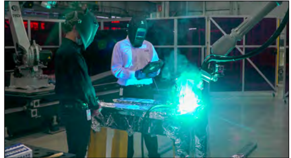
Wire Arc Additive Manufacturing is one of the innovative new processes undergoing research at LIFT. Credit: LIFT
