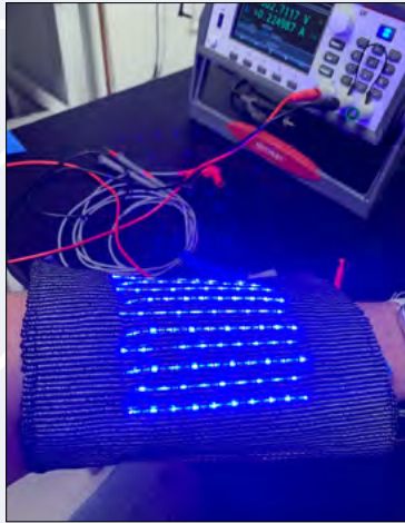
AFFOA blue LED fibers integrated into a conformal fabric for wound therapy; prototype can emit high-intensity light. Credit: AFFOA
