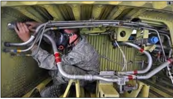
A worker inside an aircraft wing fuel tank is monitored remotely via a wearable atmospheric chemical sensor. Credit: Air Force Research Laboratory (AFRL).
