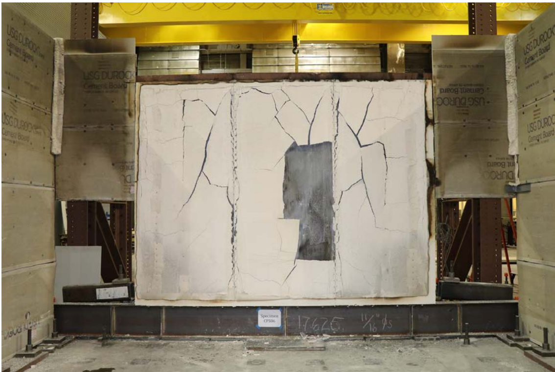
Figure 101: CFS06 – Photograph of metal sheathed side of wall after fire loading (CFS06b).
