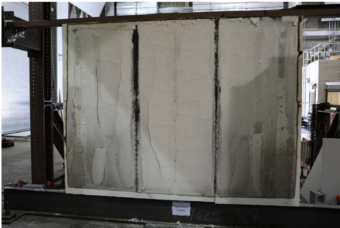
Figure 50: CFS01 - Photograph of metal sheathed side of wall after fire loading (CFS01b).
