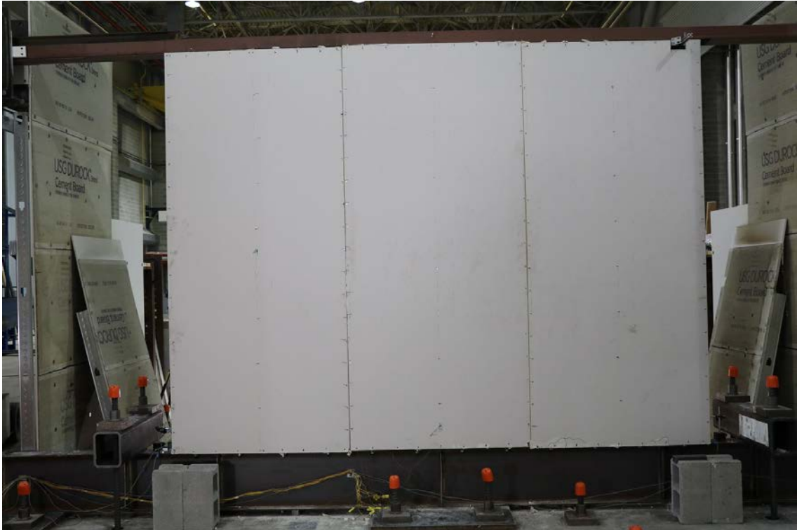
Figure 83: CFS04 – Photograph of gypsum sheathed side of wall after mechanical loading to 2.8 % drift (CFS04c).
