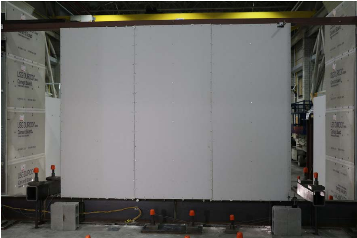
Figure 56: CFS02 - Photograph of gypsum sheathed side of wall after mechanical loading to 2.8 % drift (CFS02a).
