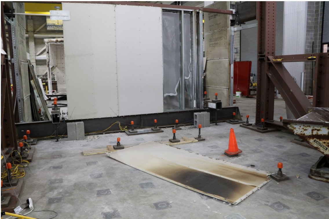
Figure 105: CFS06 – Photograph of back of metal sheathed side of wall after mechanical loading to 2.8 % drift (CFS06c) highlighting charring of gypsum board.
