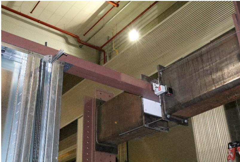
Figure 25: Photograph of string potentiometer to measure top wall drift.
