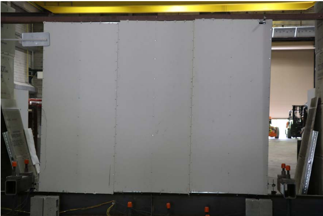
Figure 94: CFS05 – Photograph of gypsum sheathed side of wall after mechanical loading to 2.8 % drift (CFS05b).
