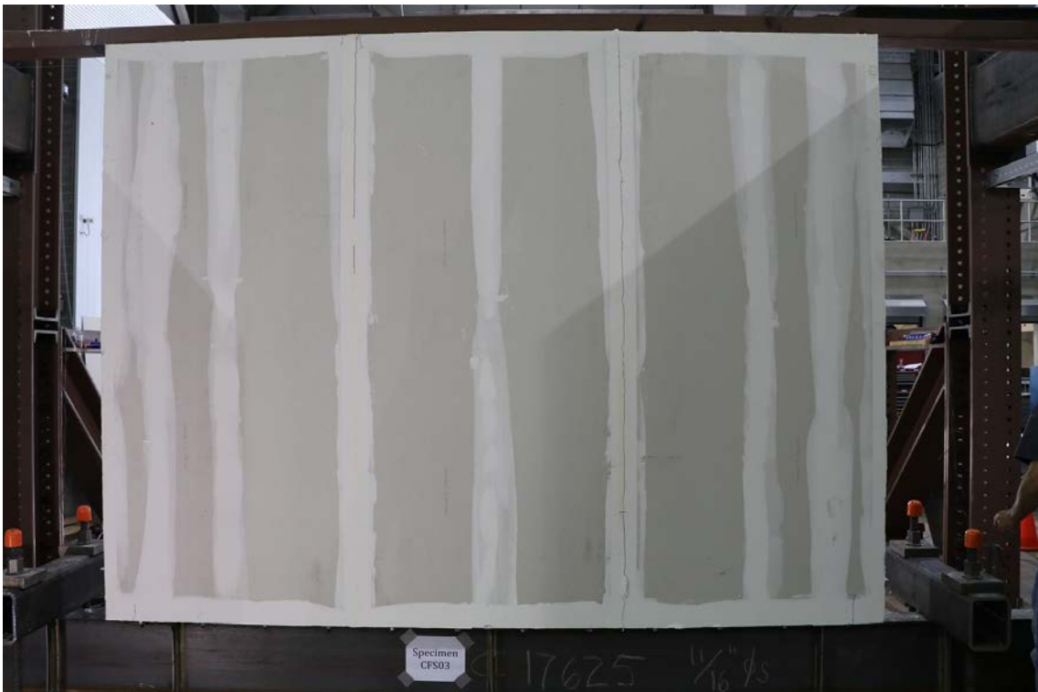
Figure 65: CFS03 - Photograph of metal sheathed side of wall after mechanical loading to 1.0 % drift (CFS03a).
