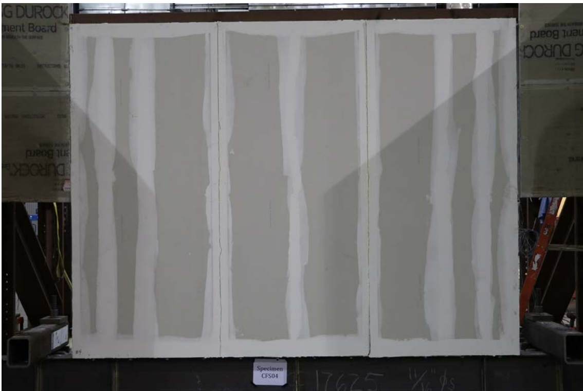
Figure 80: CFS04 - Photograph of metal sheathed side of wall after mechanical loading to 1.8 % drift (CFS04a).
