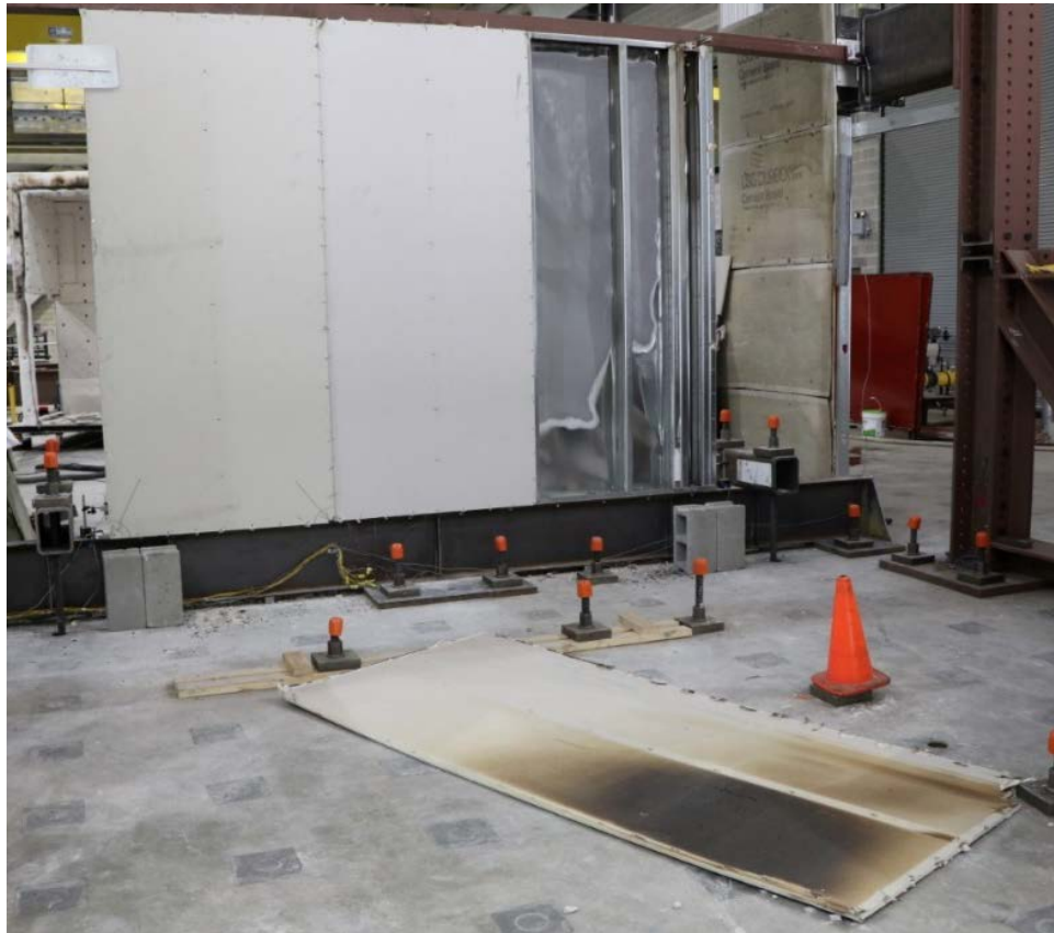
Figure 31: Photograph of back of metal sheathed side of wall after fire loading for 26m 40 s and mechanical loading to 2.8 % drift.
