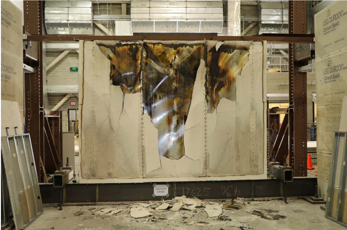
Figure 68: CFS03 – Photograph of metal sheathed side of the burned wall after mechanical loading to 2.8 % drift (CFS03c).
