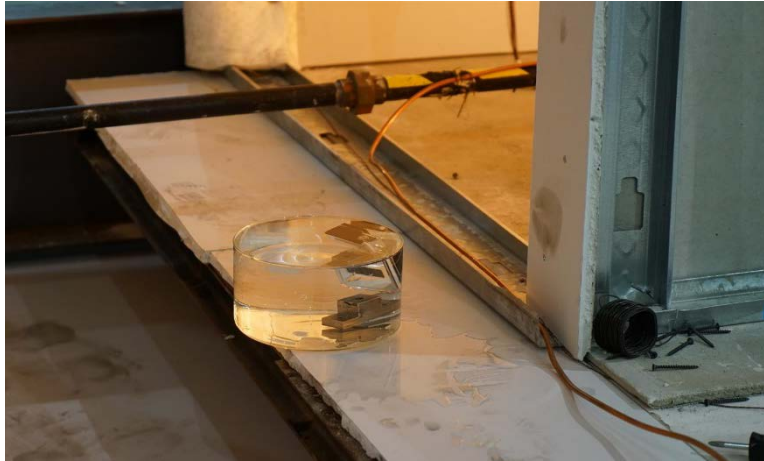
Figure 27: Photograph of GoPro video camera in water bath used to acquire footage during fire loading.
