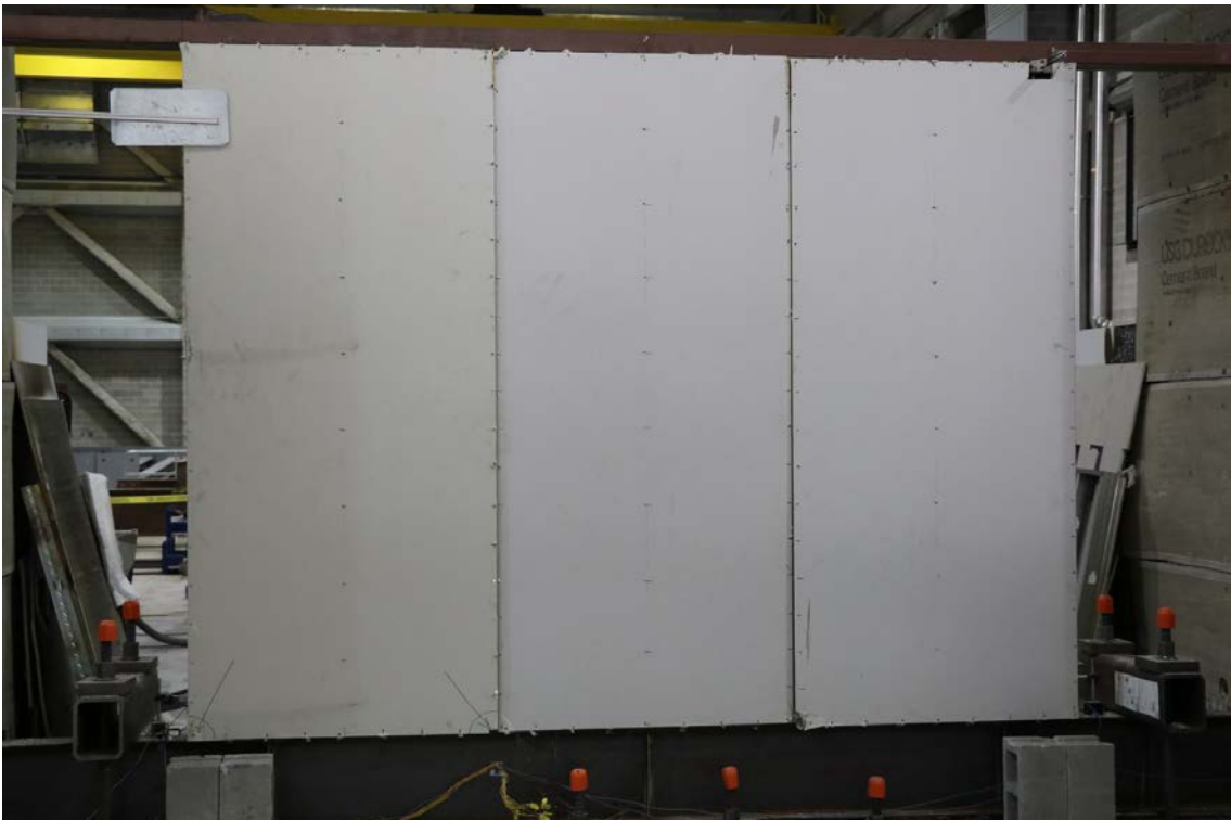
Figure 103: CFS06 – Photograph of gypsum sheathed side of wall after mechanical loading to 2.8 % drift (CFS06c).
