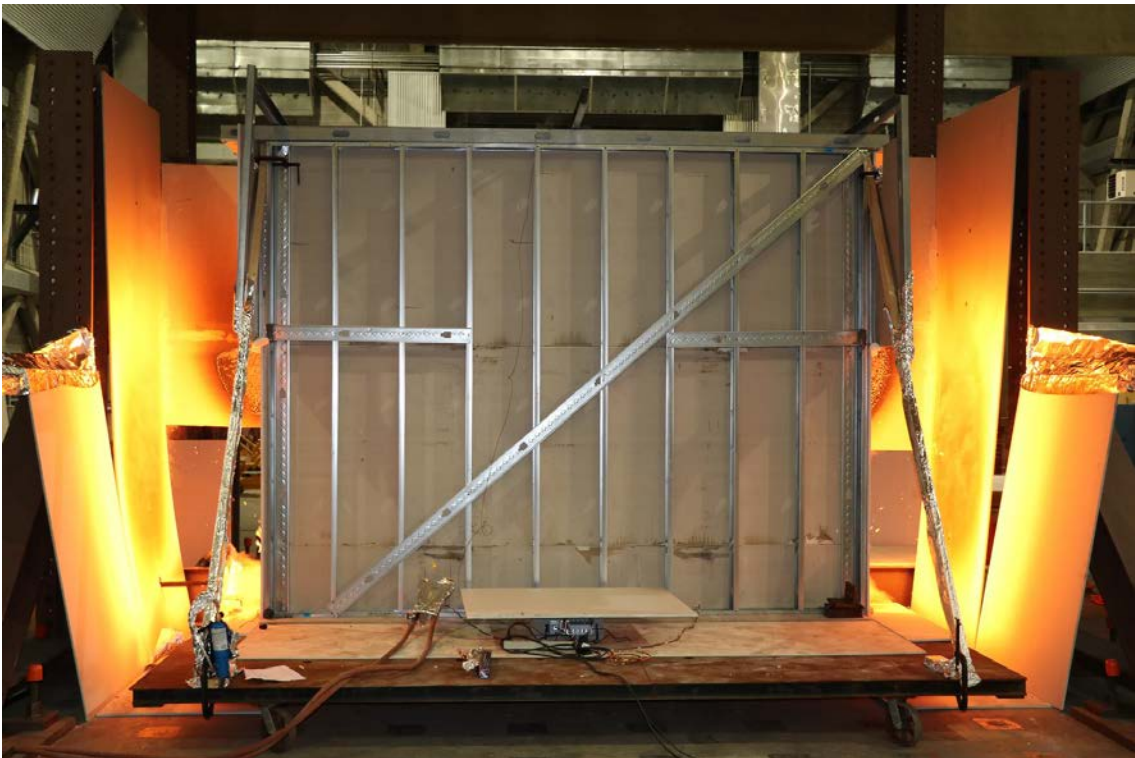
Figure 49: CFS01 - Photograph of back of compartment during fire loading (CFS01b).
