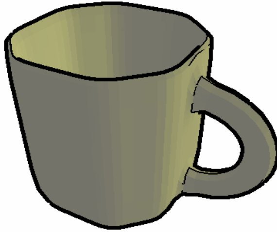
Fig. 65. Model of a cup created using both rind modeling and multi-segment curved handle tools.
