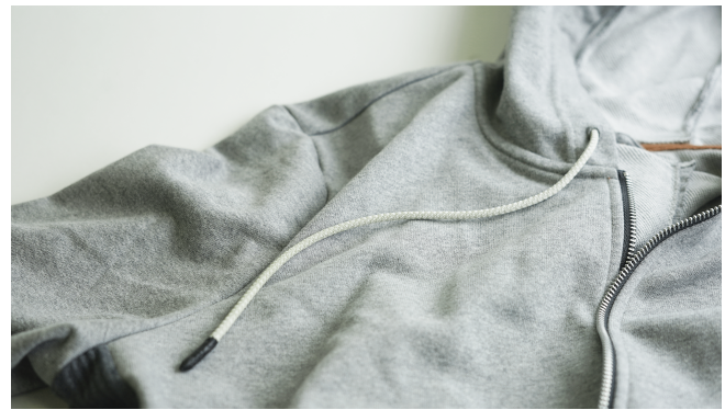
Figure 8. Hoodie with replaced left drawstring invisibly adds gesture capabilities to the garment. I/O Braid controls music playback, volume control, and switching between playlists.
