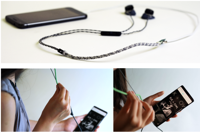
Figure 7. I/O Braid USB-C headphones with embedded gesture recognition and audio feedback for music control, enabled by Nanoboard. The user starts playback by pinching, then rolls the I/O Braid to increase the volume.
