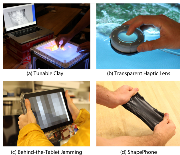
Figure 1: Jamming is a scalable technique for programmatic stiffness control, which can be applied to a variety of malleable and organic user interfaces. Examples include: Tunable stiffness for malleable interfaces on tabletops (a, c), for haptic feedback (b, c), and for mobile shape-changing interfaces (d).
