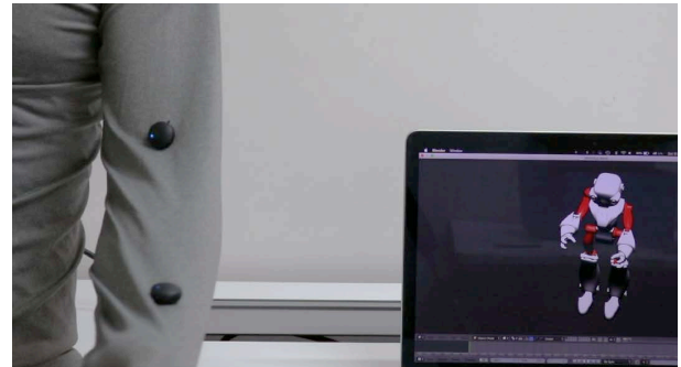
Figure 14. Multiple SensorSnaps were attached to the arm and the torso for motion tracking. The resulting 3D animation is shown on the computer screen.
