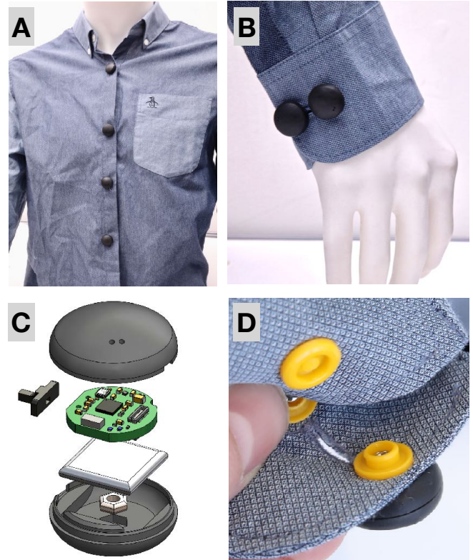
Figure 1. SensorSnaps embed miniaturized electronics into generic snap fasteners, making it possible to augment garments with wireless electronics that enable on-device gesture recognition, wireless connectivity, motion tracking with sensor fusion, and touch sensing. A) SensorSnaps replace buttons on a shirt. B) SensorSnaps are used as cufflinks. C) The exploded CAD model of a SensorSnap. The electronics and the battery are contained inside the case. D) Integration with off-the-shelf plastic snap fasteners (in yellow).
