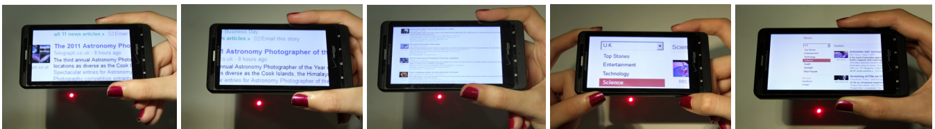
Figure 15: A participant in our informal feedback sessions zooms into a web page with the Mobile Viewport interface by varying the device's distance to the surface.
