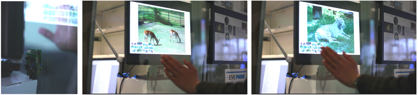
Figure 14. Low-cost motion tracking for public displays using an embedded Speckle projector and sensor (configuration D). The user's 2D hand movement selects the fullscreen image from a matrix of thumbnails in the lower left corner.
