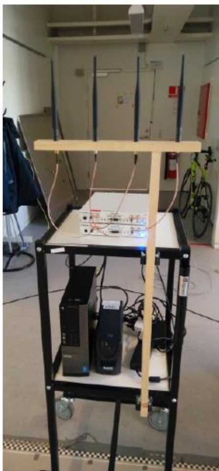
Figure 5. MIMO 4x4 node, composed of 2 USRP RIO 2953R connected to an Intel I7 host PC. Each node has an UPS which may facilitate the re-deployment in a new position without powering down the node.
