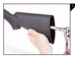
Begin by removing the existing recoil pad from your stock using a phillps head screwdriver. Next using a long flat head screwdriver or the appropriate socket with extension remove the stock bolt from the inside of the opening in the rear of the stock as seen in Figure 1.
