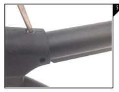
Using the provided 8-32 x 3/4" Flat Head Socket Cap Screw and a 8/32 allen wrench, tighten the buffer tube to the pistol grip as seen in Figure 5.
