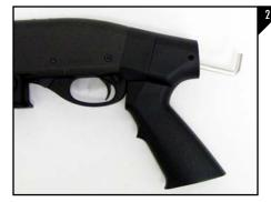
Next, place the pistol grip with the adapter onto the rear of the shotgun. Place the 1/4"- 28 x 1 1/2" bolt and supplied washer through the back of the grip and adapter and using the appropriate allen wrench secure the pistol grip to the shotgun reciever as seen in Figure 2
