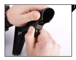
Next, grab the adjustment lever with your thumb and index finger and pull down as seen in Figure 7.
