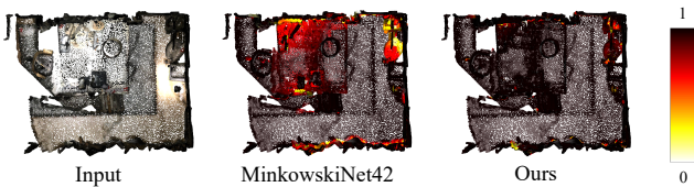
Figure 4. Heatmap visualization of consistency score (CScore). We visualize consistency scores of MinkowskiNet [6] and the proposed Fast Point Transformer with the hot heatmap. Points with high CScore (consistently predicted with the same class) are colored black, and points with low CScore (the predicted class is not consistent with arbitrary rigid transformations) are colored white. Table 1 shows the quantitative evaluation.
