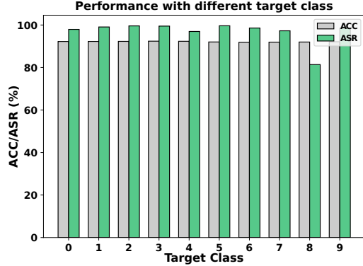
Figure 4. Effect of target class ( y_t ) on our Deep-TROJ attacking ResNet-20 trained on CIFAR-10 dataset.
