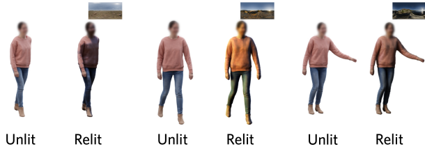
Figure 7. HDRi Relighting on MonoPerfCap using NPC [37] as the backbone. Our Gaussian relighting method can be utilized at inference with higher quality models on data that is uniformly lit.
