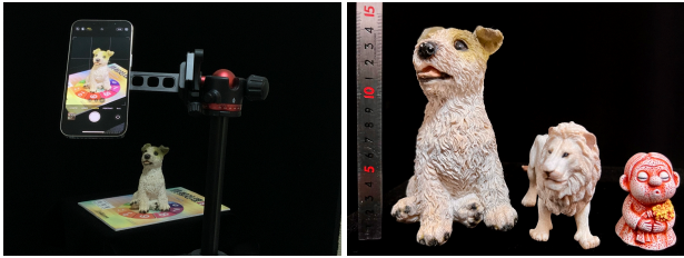
Figure 6. Our real-world data capture setup. The target object is placed on a turntable before a dark sheet under general indoor illumination. There is no need to prepare a darkroom. We use an iPhone to take images and move a video light to illuminate the object from the camera side. Objects are 6 cm to 15 cm high.
