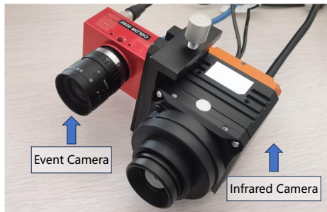
Figure 6. The hybrid camera system used to capture real data. The two cameras are temporally synchronized with a customized circuit and spatially aligned by manual keypoint matching.
