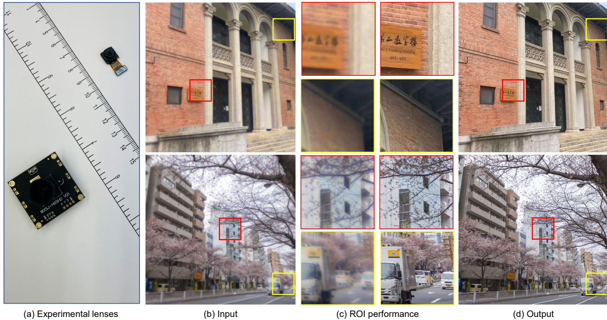
Figure 7. Results on real data captured by two compact cameras with a low-end lens. (a) The photo of two lenses, with the smaller one being only around 1cm, which is highly portable but exhibits significant aberrations. (b)(d) Raw images captured using the cameras in (a) and the results after compensation. (c) The zoomed-in view of the highlighted regions in (b) and (d), distinctly showcases the performance at both regions closer to the center (red boxes) and toward the corners (yellow boxes) of the sensor’s field of view.
