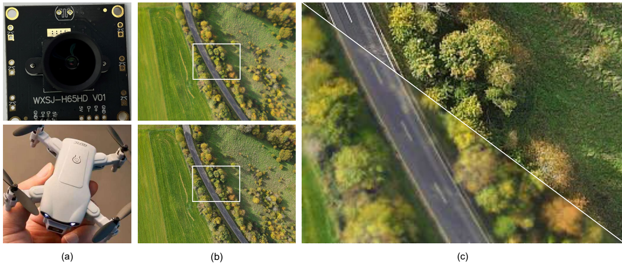
Figure 1. An illustrative example of our lens-aberration compensation approach. (a) A camera equipped with a simple lens of a large field of view but severe optical aberration (WXSJ-H65HD) and a small-sized unmanned aerial vehicle (UAV) carrying the camera for data capture. (b) The input degenerated image (upper) and our reconstruction result (lower). (c) The zoomed-in comparison on the highlighted region (white box) in (b), where the original recording is shown in the bottom left corner and the reconstructed result in the top right corner.
