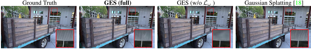
Figure 8. Frequency-Modulated Loss Effect. We show the effect of the frequency-modulated image loss \mathcal{L}_\omega on the performance on novel views synthesis. Note how adding \mathcal{L}_\omega improves the optimization in areas with large contrast or a smooth background.
