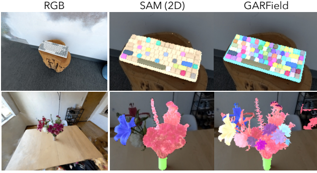
Figure 8. Segment-Anything [15] vs. GARField : SAM’s automatic mask generator may struggle with recalling all masks, especially when there are clusters of small masks and the camera is far away from the object. In contrast, GARField’s scale-conditioned affinity field incorporates masks from multiple viewpoints in 3D.
