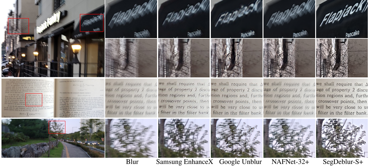
Figure 6. Visual comparison results on real-world blur images. NAFNet-32+ and SegDeblur-S+ are the accelerated (faster) models for the deployment and they are evaluated for fair comparison with the commercial applications. This will be more discussed in Section 4.4.
