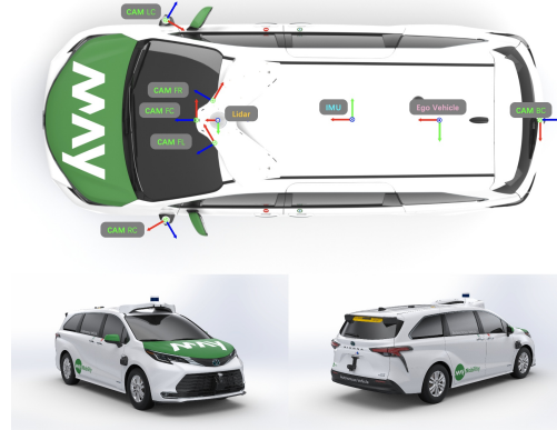
Figure 2. Sensor setup of the vehicle platform for data collection.
