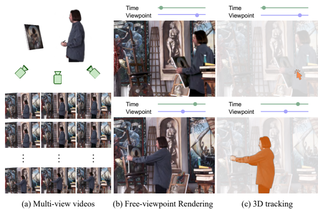
Figure 1. (a) Our method takes RGB videos captured from a camera array as input. (b) Trained Gear-NeRF achieves photo-realistic real-time free-viewpoint rendering of a dynamic scene. (c) With users giving a single click at any time and from any viewpoint, our method can perform free-viewpoint tracking of the target object.
