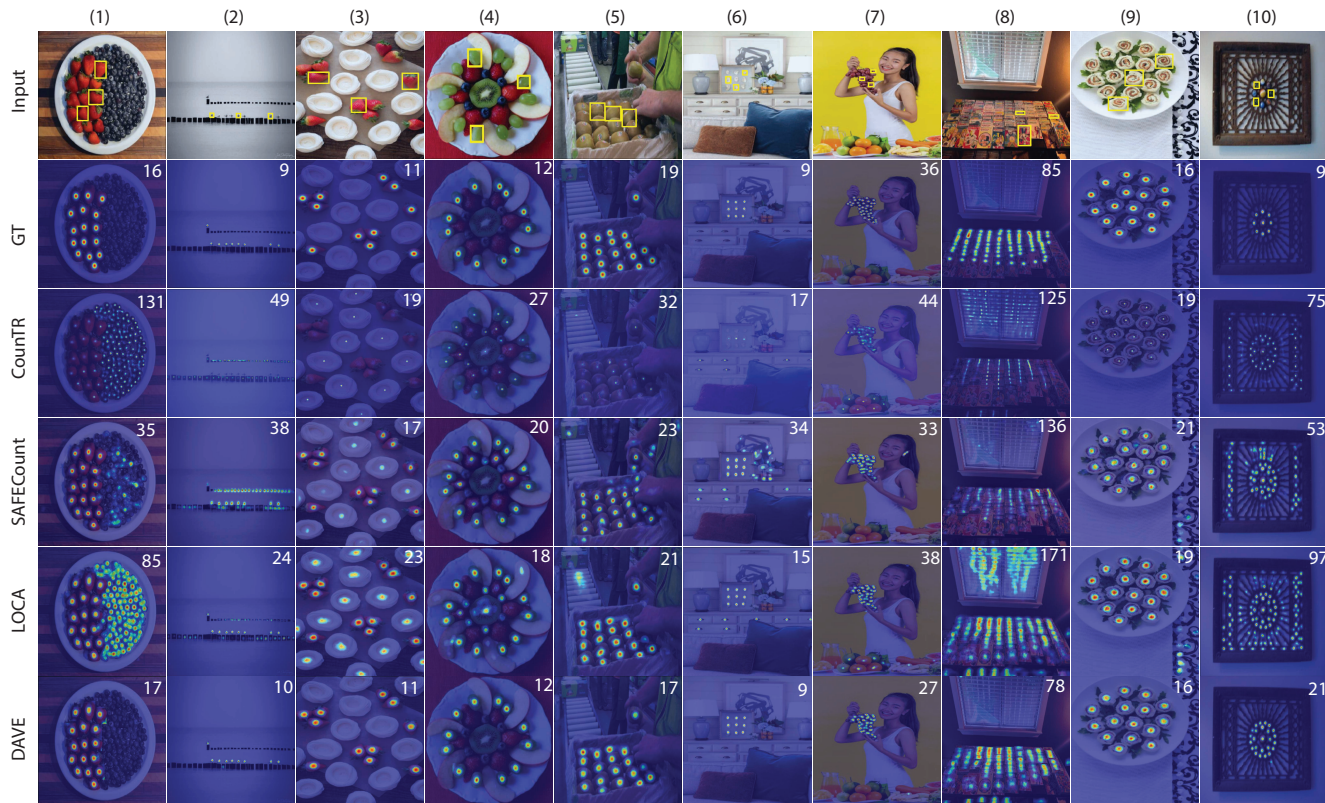
Figure 3. Qualitative comparison of DAVE with LOCA [6], SAFECOUNT [38] and CountR [16]. The first two columns show the input images and the ground truth (GT), while the predicted densities are shown in the rest.
