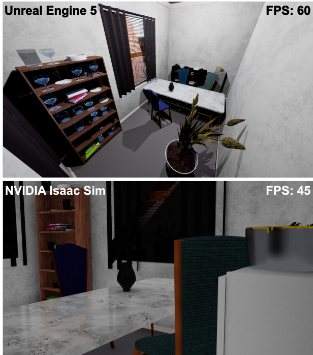
Figure 12. A single scene from two different viewpoints in Unreal Engine 5 (above) and Omniverse Isaac Sim (below). Unreal Engine runs at 60 FPS and Isaac Sim with physics simulation enabled runs at 45 FPS, both on RTX 3090s. Differences in lighting are caused by the variations in simulator import systems.
