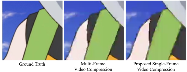
Figure 7. H.264 [31] compression of regular multi-frame video compression and our proposed single-frame compression. They exert similar degradations ( e.g. , distortion to hand-drawn lines).
