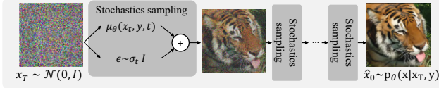
(a) The inference of SR3 [33] starts from a pure noise, which requires a large number of inference steps (T=100 after using DDIM [37]).
