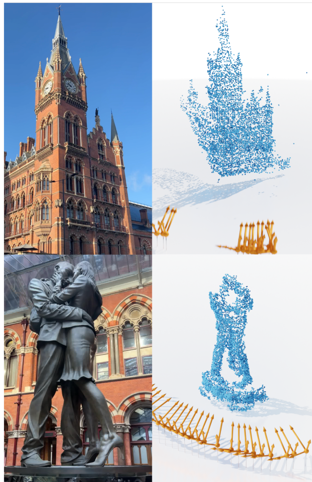
Figure 1. Reconstruction of In-the-wild Photos with VGGSfM , displaying estimated point clouds (in blue) and cameras (orange).
