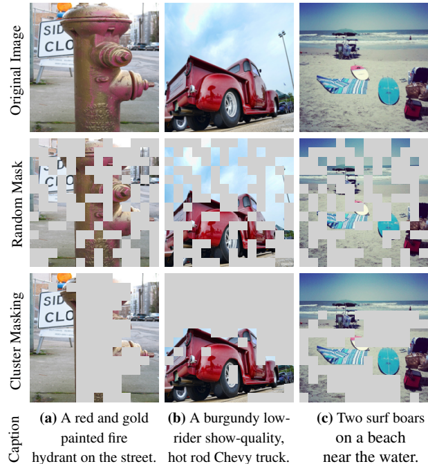
Figure 1. Cluster masking. We mask random clusters of visually similar image patches when training contrastive vision-language models (bottom). This masking strategy distinguishes our approach from methods that independently mask image patches for efficiency [36] (middle), while providing a similar improvement in training speed. It provides an extra learning signal, since it forces a model to predict words for missing scene structures solely from context.
