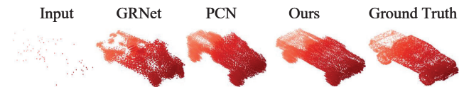
Figure 1. We use 64 points as input for point cloud completion. The PCN [57] result does not result in good general shapes. GRNet [51] result has unexpected holes due to the lack of dense representations. In comparison, our few-point shape completion method can provide much more reasonable results.
