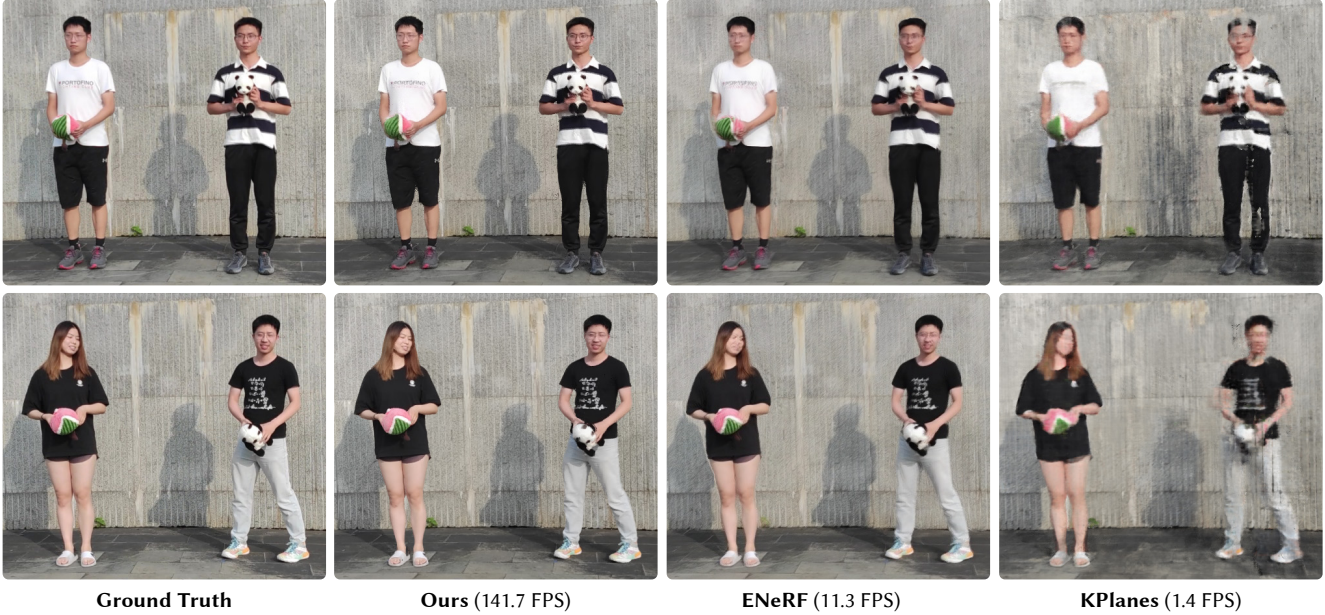
Figure 3. Qualitative comparison on the ENeRF-Outdoor [49] dataset that contains 960 \times 540 images. Our method achieves much higher rendering quality and can be rendered 14\times faster than ENeRF[49]. More dynamic results can be found in the supplementary video.
