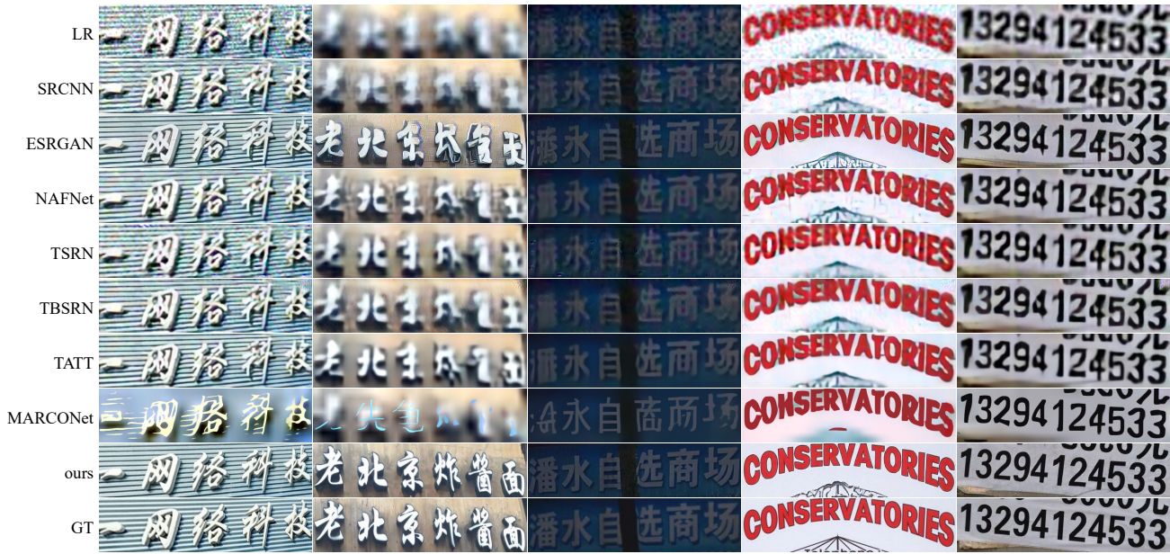
Figure 4. Qualitative comparison for the synthetic dataset CTR-TSR-Test with different methods including SRCNN [7], ESRGAN [43], NAFNet [5], TSRN [42], TBSRN [3], TATT [25], MARCONet [23] and our method for \times 4 super-resolution.
