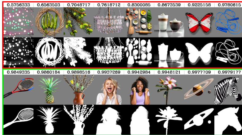
Figure 18. Automatic selection: Randomly generated images with similarity scores increasing from left to right. The top 50%, highlighted in green, are kept while the rest are discarded. Samples with high similarity almost always have accurate alpha mattes.
