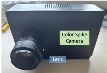
Figure 1. The color spike camera we used in the experiments to capture real-world Bayer-pattern spike stream.
