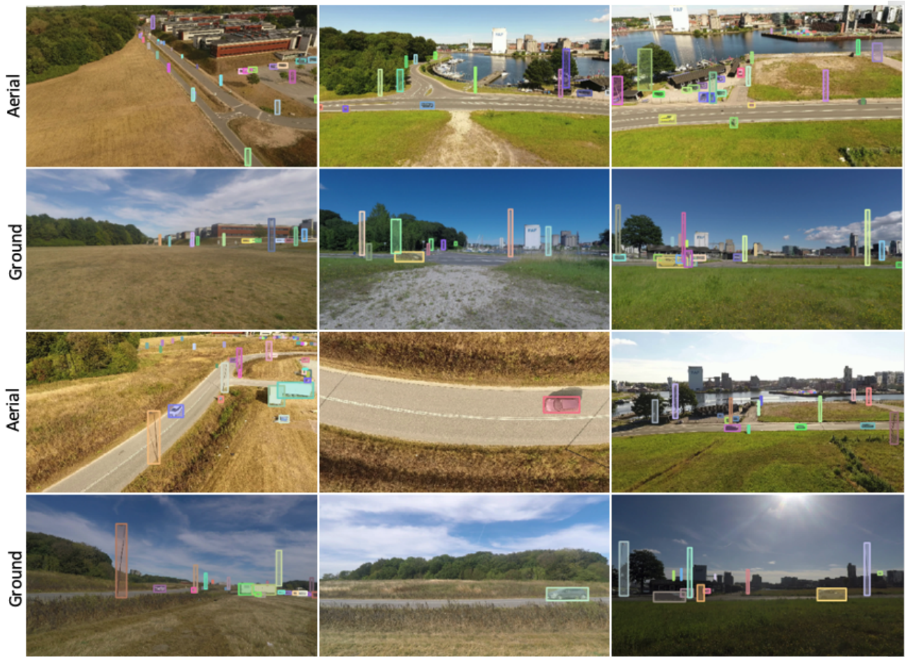
Figure 9. Different sample scenes (with annotation) from our dataset; the first row is the aerial view, and the second row presents the same scenes from a ground camera. Similarly, the third row is the aerial view, and the fourth row presents the same scenes from a ground camera. Some scenes have dense object annotations, while some scenes have very few object annotations. This high variance in object distribution across different scenes in MAVREC is complementary to datasets like VisDrone [91] where object detection is relatively straightforward due to their biased object distribution (dense), reflecting its demographic characteristics.
