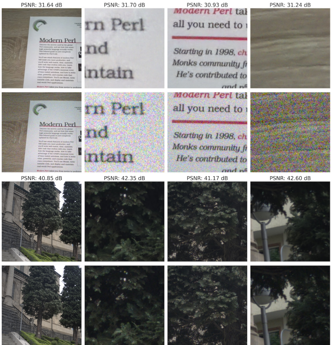
Figure 6. Qualitative evaluation of images denoised using the SplitterNet trained on the MIDD. The first and third rows, denoised images obtained with our model are presented as well as their PSNR scores. The original noisy input images are shown in the second and fourth rows. The first two rows show an indoor scene with strong noise. The model extracts the noise very well on the wooden surface, as seen in the fourth column, but introduces some artifacts when denoising the letters on the book surface. The second scene shows a daylight image with very little noise. Our model does not over-smooth edges and only minor changes are made by the model.
