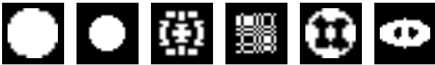
Figure 3. Coded apertures considered for ablations. We test out various coded apertures in conjunction with dual-pixel sensors in simulations. From left to right, showing no code mask, no code (50% size) mask, Levin et al. [8] mask, separable MLS code [15], Shedligeri et al. [11] mask, and our proposed end-to-end learned CADS mask.
