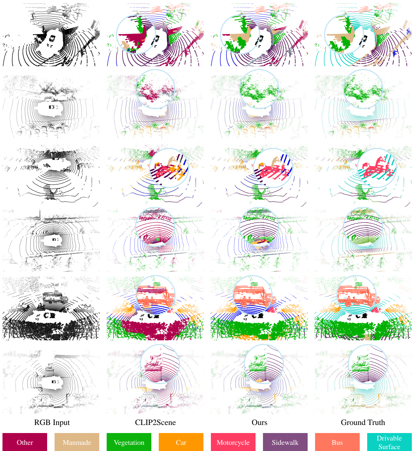
Figure 4. Qualitative comparison for semantic segmentation of our method and CLIP2Scene [2] on the nuScenes dataset.
