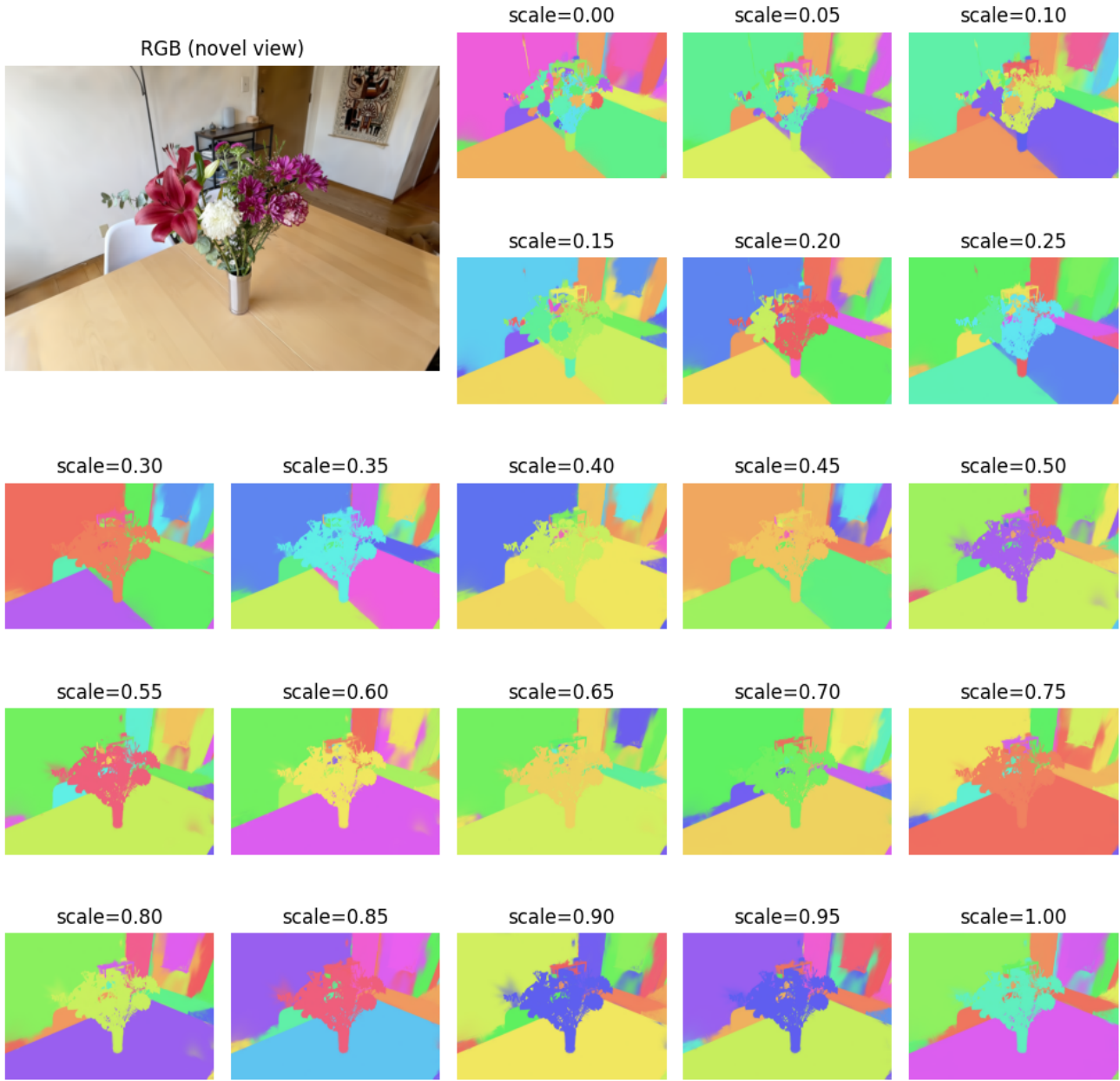
Figure 14. Global Clustering Results (“Bouquet”) : Global clusters at smaller scales ( s = 0 ) distinguish between different sections of the bouquet, as well as the two halves of the table. At a larger scale, the bouquet and table are considered whole.
