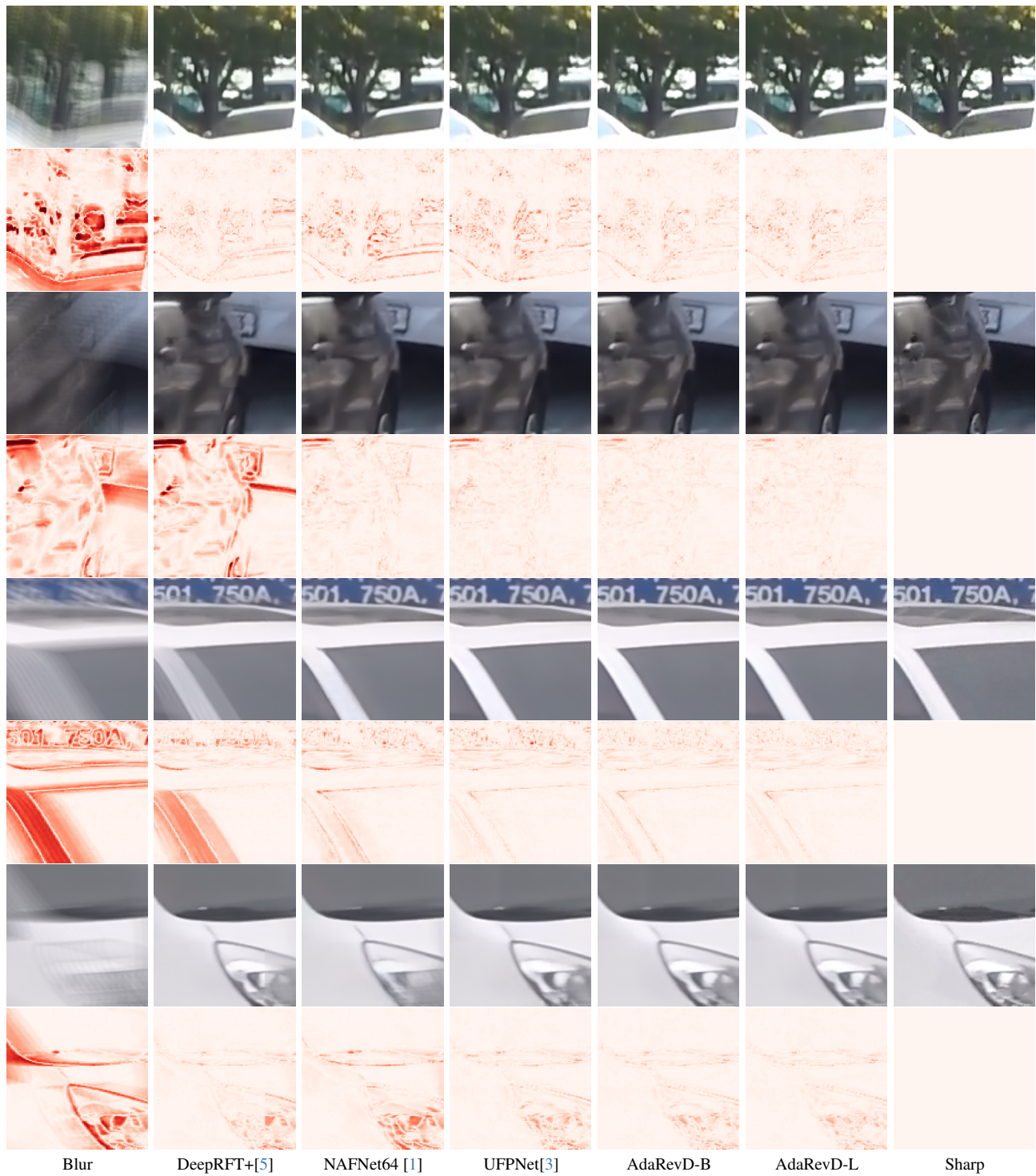
Figure 4. Examples on the GoPro test dataset. The odd rows show blur image, predicted images of different methods, and ground-truth sharp image. The even rows show the residual of the blur image / predicted sharp images and the ground-truth sharp image.
