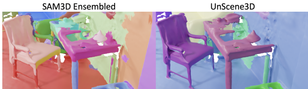
Figure 3. While SAM has powerful capabilities in crisp 2D mask generation, when aggregated on 3D, SAM3D tends to over-segment object instances.
