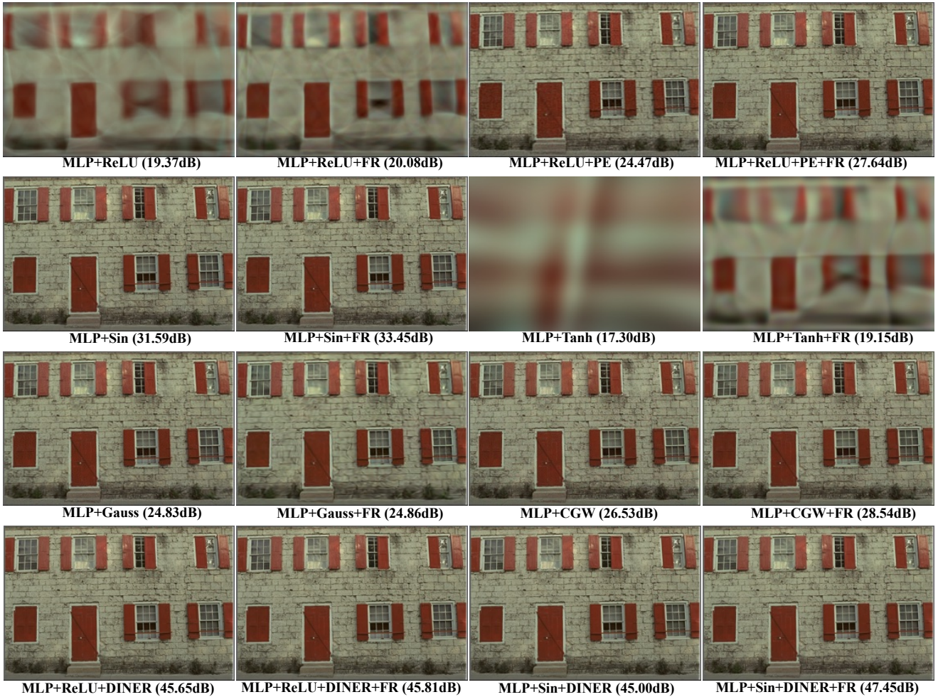
Figure 2. Peak signal to noise ratio (PSNR) of 2D color image approximation results on Kodim 01. MLP+Gauss denotes the MLP with Gauss activation function [5]. MLP+CGW denotes the MLP equipped with complex Gabor wavelet activation function [6]. MLP+ReLU+DINER denotes the MLP+ReLU coupled with the adjusted input features by a hash-table [8]. Detailed experiment settings can be found in Section 5.1 and Appendix E.
