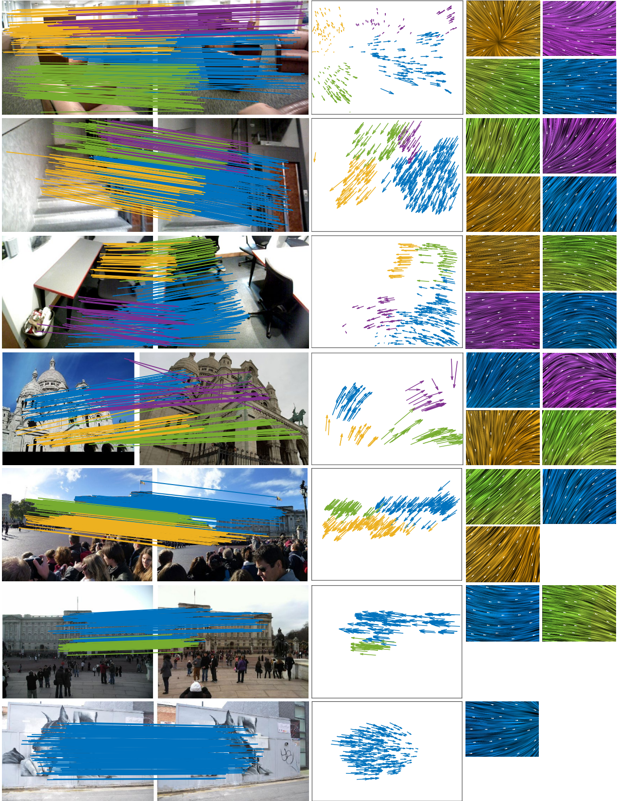
Figure 6. Illustration for piecewise smoothness property. Clusters are marked with different colors to represent different motion patterns, and the sub-field is formed by the cluster that is painted with a similar color. Zoom in for better visualization.
