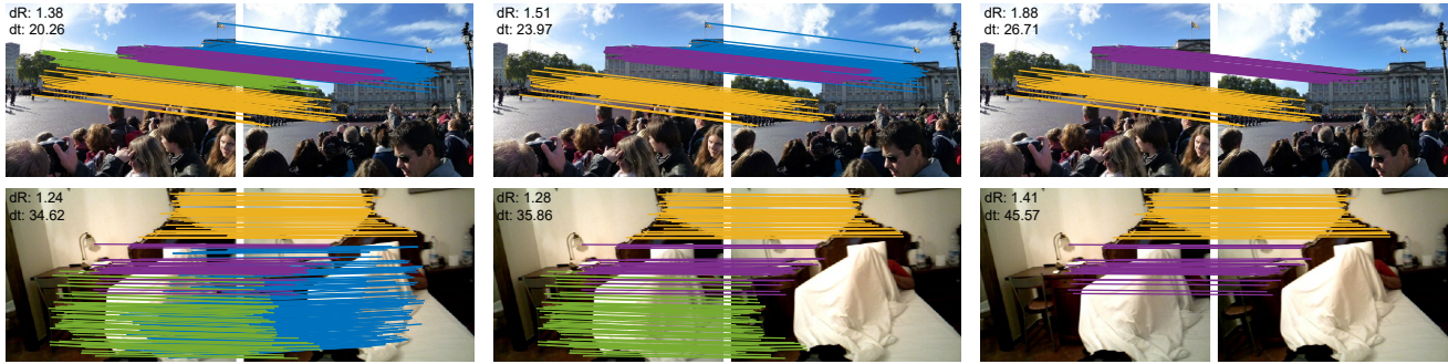
Figure 7. The effect of sub-fields on the final performance. Motion clusters that form smooth sub-fields are removed gradually. The errors of rotation and translation are shown in the top-left corner. Zoom in for better visualization.
