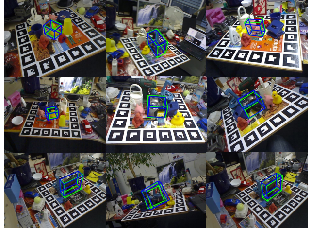
Figure 8. Visualization of 6D pose estimation for unseen objects on LINEMOD [15]. The ground-truth 6D object pose and the predicted pose in the query image are depicted as green and blue 3D bounding boxes, respectively.
