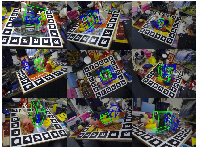
Figure 9. Failure cases of 6D pose estimation for unseen objects on LINEMOD [15].
