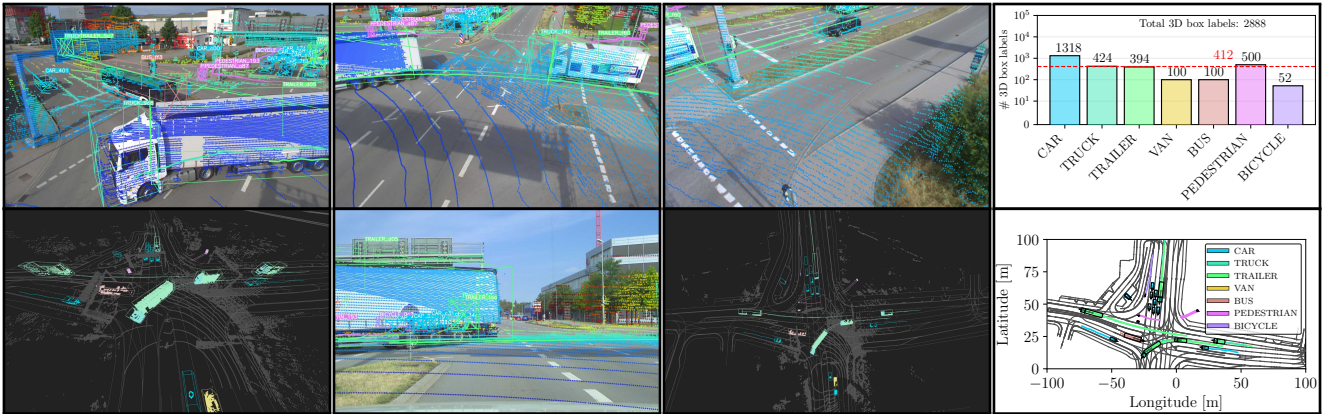
Figure 8. Visualization of drive_26 of the TUMTraF-V2X dataset. In this drive, multiple trucks and trailers occlude traffic participants. These traffic participants are visible from the elevated roadside cameras and LiDAR mounted on the infrastructure. This sequence contains 2,888 labeled 3D objects.
