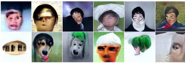
Figure 6: Images synthesized to activate a hidden neuron (number 196) previously identified as a “face detector neuron” [64] in the fifth convolutional layer of the AlexNet DNN trained on ImageNet. The PPGN uncovers a large diversity of types of inputs that activate this neuron, thus performing Multifaceted Feature Visualization [40], which sheds light into what the neuron has learned to detect. The different facets include different types of human faces (top row), dog faces (bottom row), and objects that only barely resemble faces (e.g. the windows of a house, or something resembling green hair above a flesh-colored patch). More examples and details are shown in Figs. S19 & S20.
