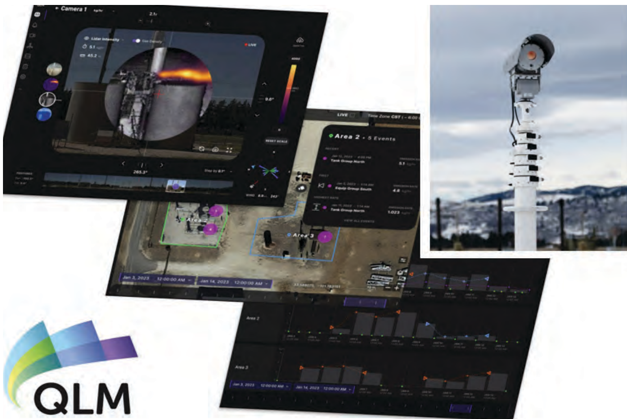
QLM Cloud analytics portal showing lidar viewfinder, emissions map and emissions event trending and reporting (left). QLM Quantum Gas Lidar system hardware (right).
