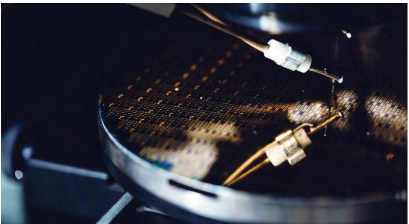
Kudos for Kubos: A 150-mm wafer of GaN LEDs under test via wafer probing.
